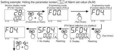
Even if hidden, the parameters of Parameter setting mode will appear (and the settings can be changed) in Engineering mode.
