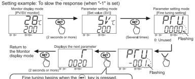
If the set value of Fine tuning is returned to "0: Unused," Fine tuning correction will no longer be applied to control.
