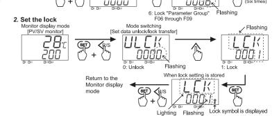
The Set lock level (Lock) settings can be changed after lock is executed.
